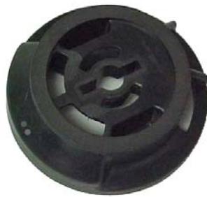
Old Distributor (Shiny Black color) - Teflon Impregnated Molded Resin Material. 0 - 1 Bumps
